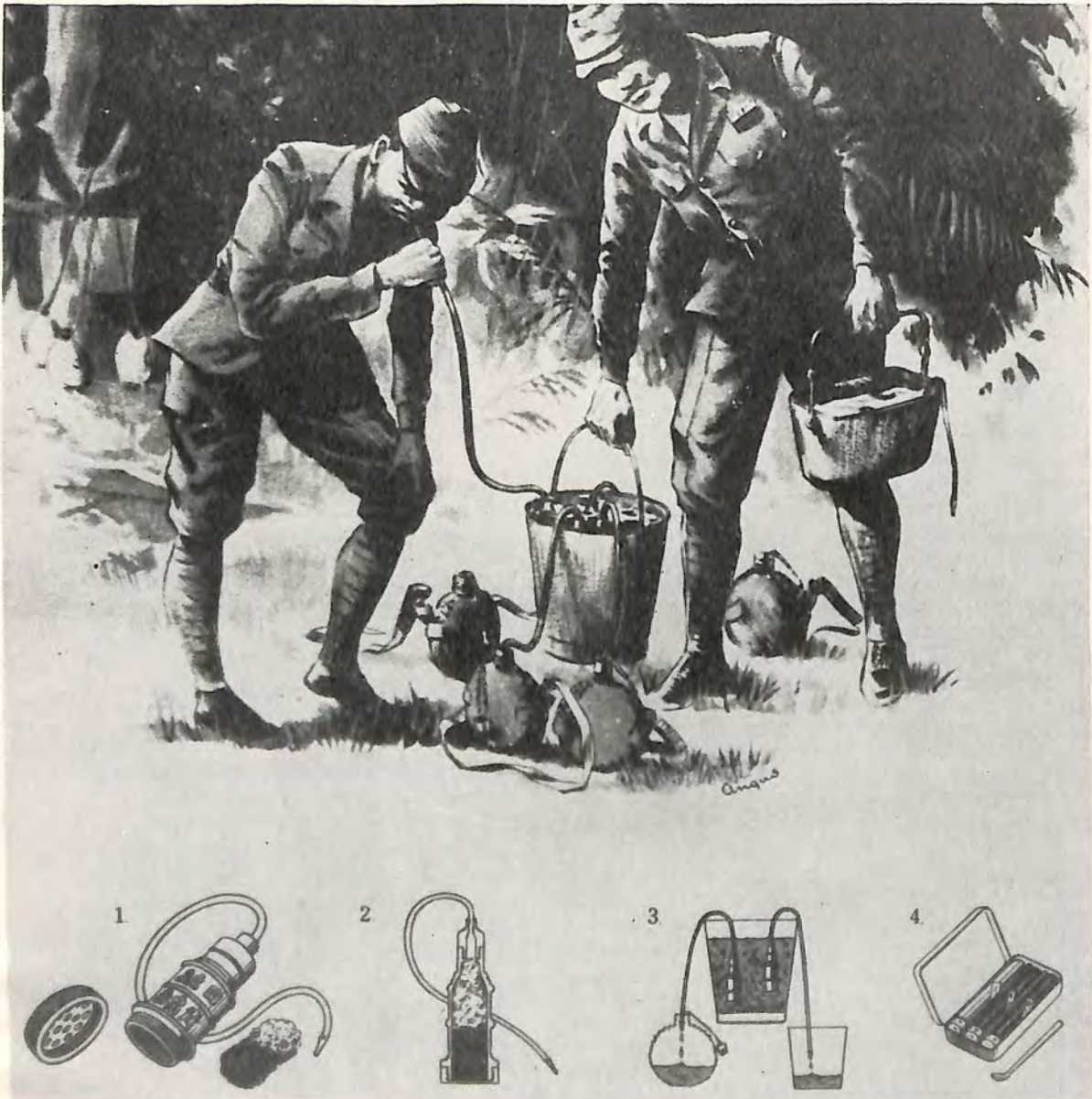
Figure 412. (Above) Japanese troops using the water filter purifier. (Below) illustrations showing components and methods of operation.
